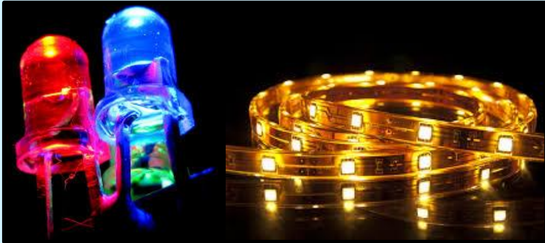
Fig. 1: LED Lamps and LED Strips
